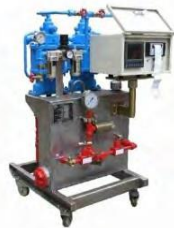
BOP Test Unit
